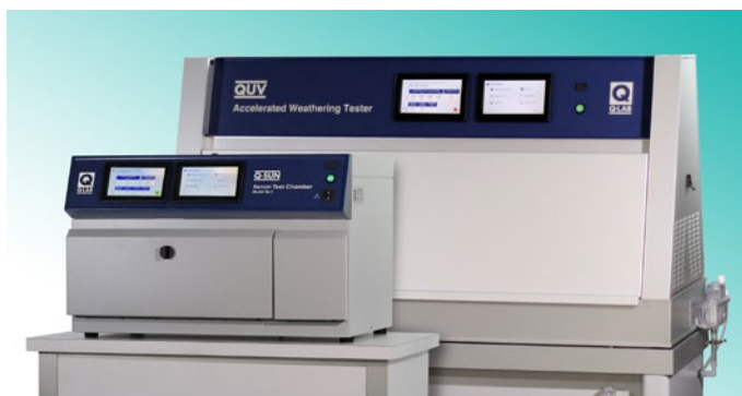
The Q-SUN Xe-1 xenon arc chamber and QUV Accelerated Weathering Tester, can both be found in Elastocon's testing laboratory.
