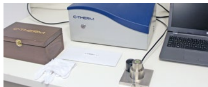
TCi is a thermal conductivity meter from the Canadian company C-Therm.
