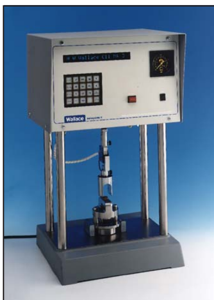
Figure 4 Stress relaxation system for discontinuous measurements using jigs
