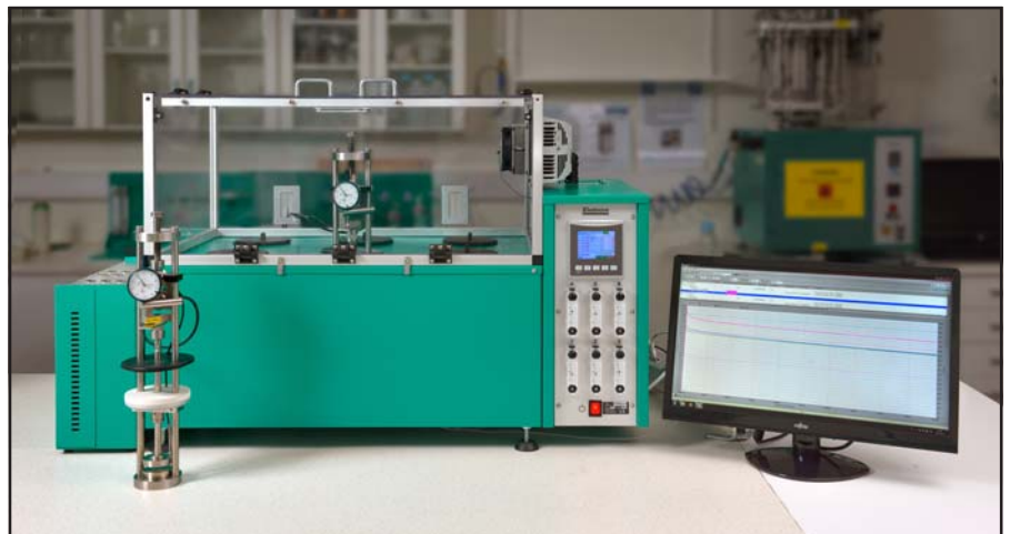
Figure 2 Relaxation rigs in a cell oven
