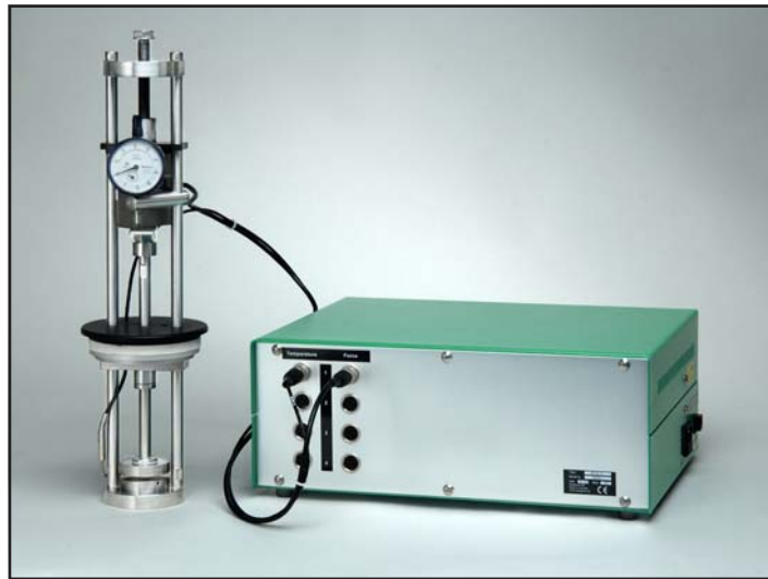
Figure 1 Stress relaxation system for continuous measurements
